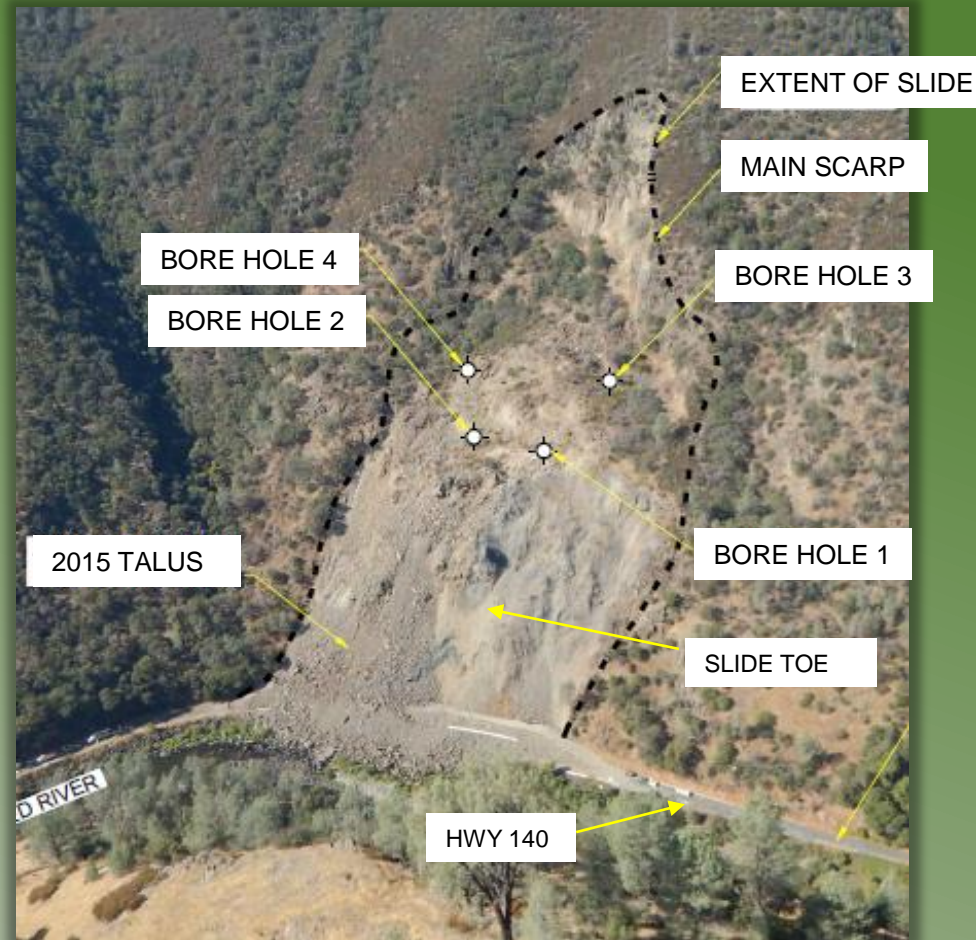
Photo: Extent of rock slide illustrating head scarp, toe, mass, talus of slide and bore hole locations.
